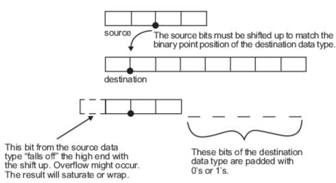
As the diagram shows, the source bits are shifted up so that the binary point matches the destination binary point position. The highest source bit does not fit, so overflow might occur and the result can saturate or wrap. The empty bits at the low end of the destination data type are padded with either 0's or 1's:
